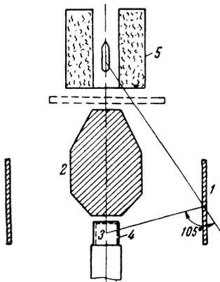
FIG. 2. Schematic of experimental arrangement: 1 – scatterer, 2 – lead cone, 3 – NaI(Tl) crystal, 4 – screen (1.5 mm Pb), 5 – furnace with source.
