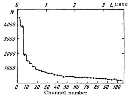
FIG. 2. Time distribution of electrons from  $\mu^-$ -meson decay in a Fe+Al target. Here and throughout  $N$  is the sum of the counts in the three analyzer channels.
