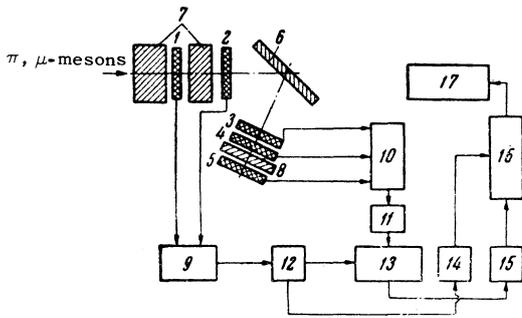
FIG. 1. Block diagram of setup: 1–5 (scintillation counters); 6 – target; 7 – copper absorbers; 8 – aluminum absorber; 9, 10 – coincidence and anticoincidence block; 11 – delay; 12 – gate duration flipflop; 13 – gate; 14–15 – shaping devices; 16 – converter; 17 – pulse height analyzer.
