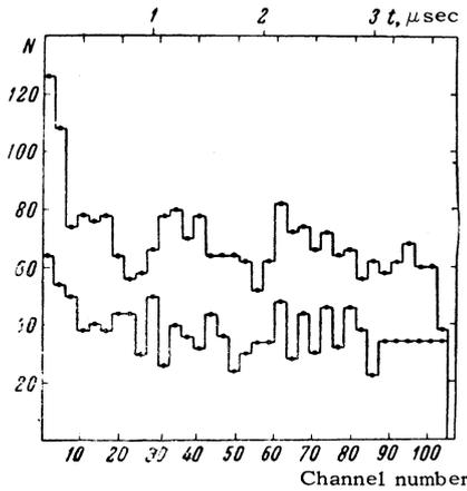
FIG. 4. Time distribution of 4 + 5 - 3 anticoincidence pulses for Zn + Al (upper histogram) and Fe + Al (lower histogram) targets.
