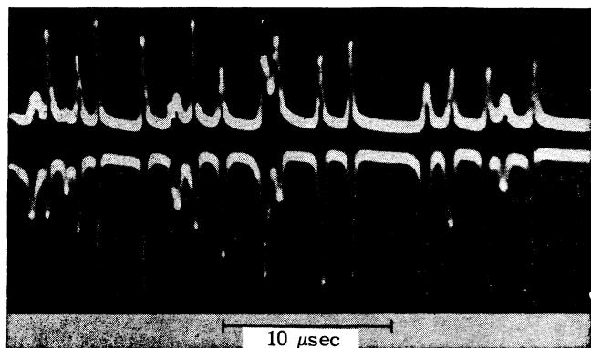
FIG. 1. Oscillogram of the emission from two sections of the end face of a ruby laser crystal.
