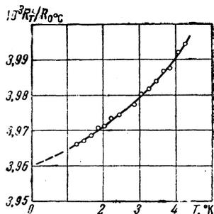
FIG. 1. Temperature dependence of the electrical resistance of iron with the earth's field compensated.
