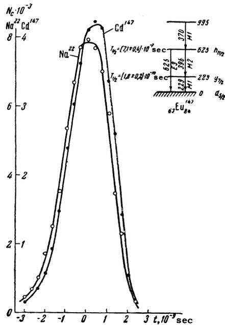
FIG. 1. Coincidence curves (one of six series) for sources of  $Gd^{147}$  (decay scheme shown in insert) and  $Na^{22}$ , taken with a pair of NaI (Tl) crystals with the same energy intervals.
