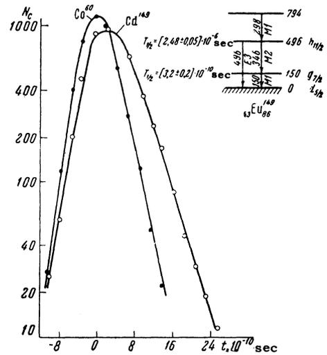
FIG. 2. Coincidence curves (one of five series) for  $Gd^{149}$  and  $Co^{60}$  sources, taken with a pair of stilbene crystals.
