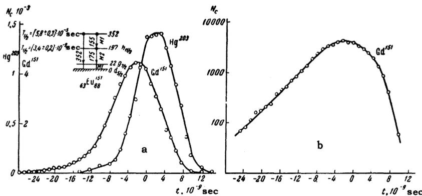
FIG. 4. Coincidence curves for  $Gd^{151}$  and  $Hg^{203}$  sources, taken with the energy intervals shown in Fig. 3, in ordinary (a) and logarithmic (b) scale. The source was deposited on a  $10\mu$  thick aluminum backing, which freely transmits the K conversion electrons of the 175-keV line.
