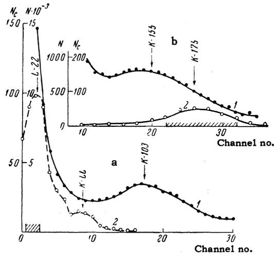
FIG. 3. Spectrum of conversion electrons from a  $Gd^{151} + Gd^{153}$  source. a) region of the 21.7-keV transition: 1) singles spectrum, 2) spectrum of electrons coincident with the K line of 175 keV; b) region of the 175-keV transition: 1) singles spectrum, 2) spectrum of electrons coincident with the 21.7 keV L conversion line for a delay of 20 nsec. The cross-hatching on the abscissa shows the position of the "windows" of the pulse analyzers in the time measurements.
