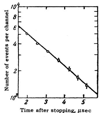
FIG. 4. Temporal distribution of decay positrons.
