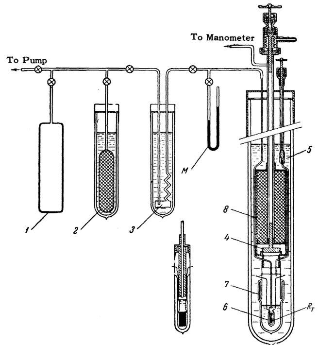
FIG. 1. Diagram of system and apparatus for determination of  $T_\lambda$  (see description in text).
