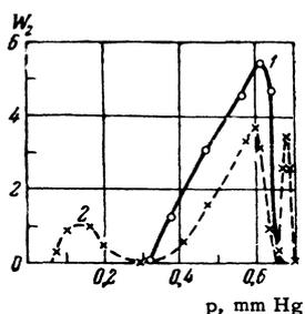
FIG. 2. Dependence of the power  $W_2$  radiated in the second cavity on the voltage  $V$  on the sorting system and on the ammonia pressure  $p$  in the beam source: curve 1 -  $V = 4.5$  kV, 2 -  $V = 8$  kV
