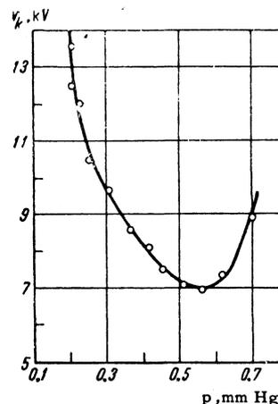
FIG. 3. Dependence of the voltage  $V_k$ , at which  $W_2 = W_2(V) = 0$ , on the pressure  $p$  in the molecular-beam source.
