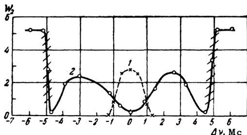
FIG. 1. Dependence of the radiation power  $W_2$  in the second cavity as the detuning  $\Delta\nu_1 = \nu_1 - \nu_{21}$  of the first cavity is varied, for two values of the sorting-system voltage: 1 -  $V = 4.5$  kV, 2 -  $V = 8$  kV.
