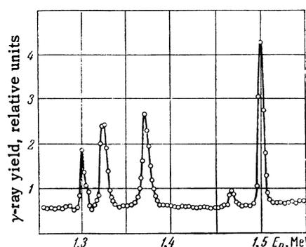
FIG. 1. Relative yields of  $\gamma$  rays from the reaction  $\text{Si}^{29}(\text{p}, \gamma)\text{P}^{30}$
