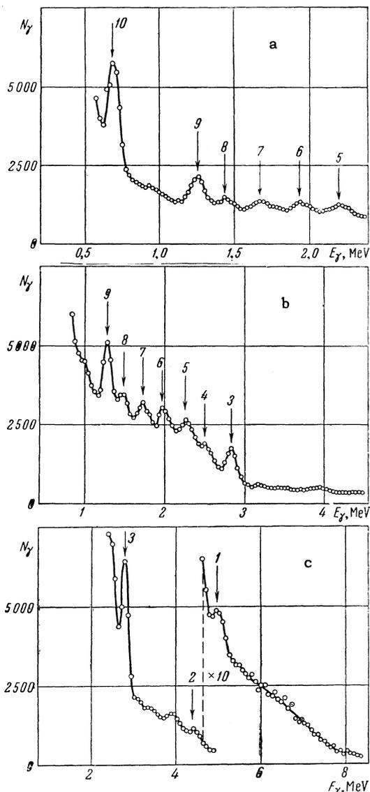
FIG. 4. Spectrum of  $\gamma$  rays from  $\text{Si}^{29}(p, \gamma)\text{P}^{30}$  in the resonance at  $E_p = 1500$  keV. a – soft portion of spectrum, b – intermediate portion, c – hard portion.
