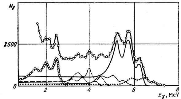
FIG. 3. Hard portion of the spectrum shown in Fig. 2, after subtracting the  $\gamma$ -ray background measured at the base of the resonance. The top curve through the experimental points is the measured spectrum. The dashed, dotted, continuous, and dot-dash curves represent  $\gamma$  lines resulting from the analysis of the measured spectrum.
