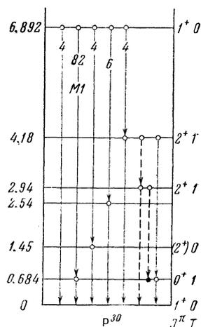
FIG. 5. Decay scheme and  $\gamma$  transitions from the 6.892-MeV  $\text{P}^{30}$  resonance level.
