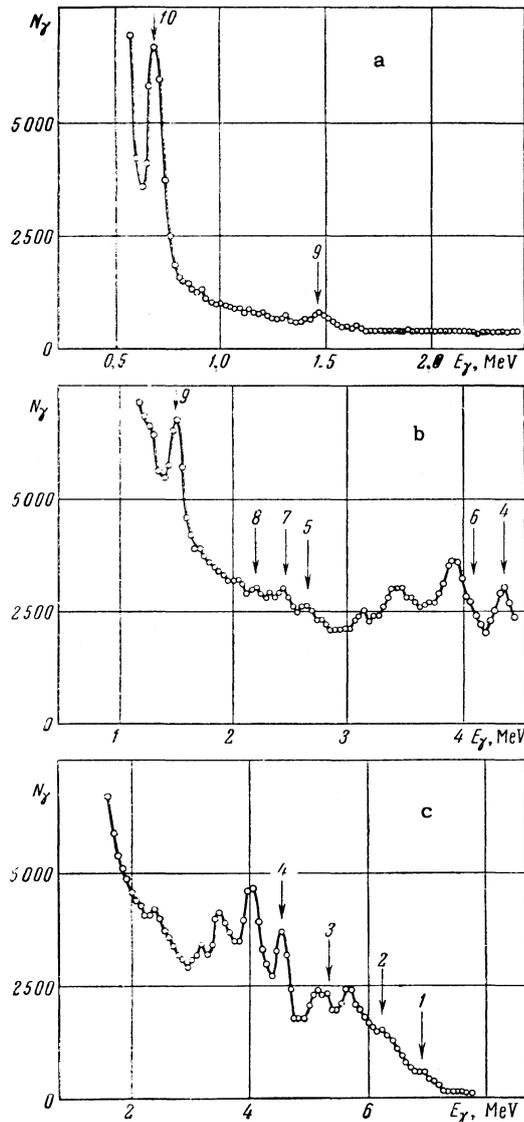
FIG. 2. Spectrum of  $\gamma$  rays from  $\text{Si}^{29} (p, \gamma) \text{P}^{30}$  in resonance at  $E_p = 1375$  keV. a — soft portion of spectrum, b — intermediate portion, c — hard portion.
