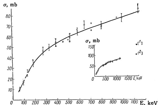
The cross section of the T + T reaction as a function of tritium energy E.
