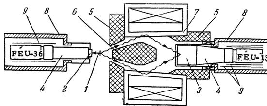
FIG. 1. Experimental layout. 1—Source; 2—stilbene crystal; 3—NaI (Tl) crystal; 4—light pipe; 5—lead collimator; 6—lead shield; 7—analyzing magnet; 8—Armco-iron shield; 9—perm-alloy shield.
