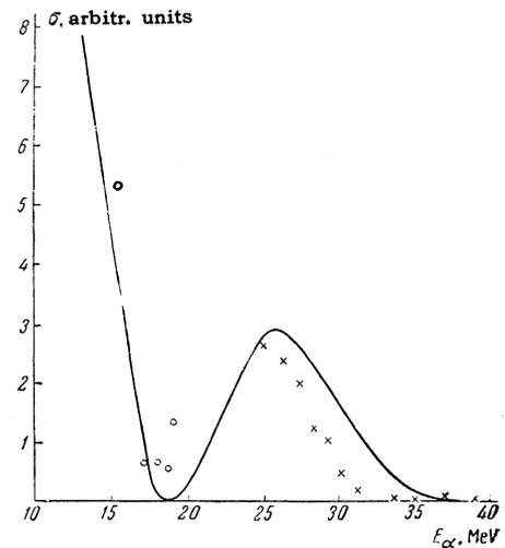
FIG. 1. Dependence of the cross section at 180° (solid curve) on the  $\alpha$ -particle energy for the  $C^{12}(\alpha, p)N^{15}$  reaction ( $R_0 = 6F$ ,  $\rho_0 = 5F$ ). The experimental points refer to the angle 170° (o - from <sup>[5]</sup>, x - from <sup>[4]</sup>).
