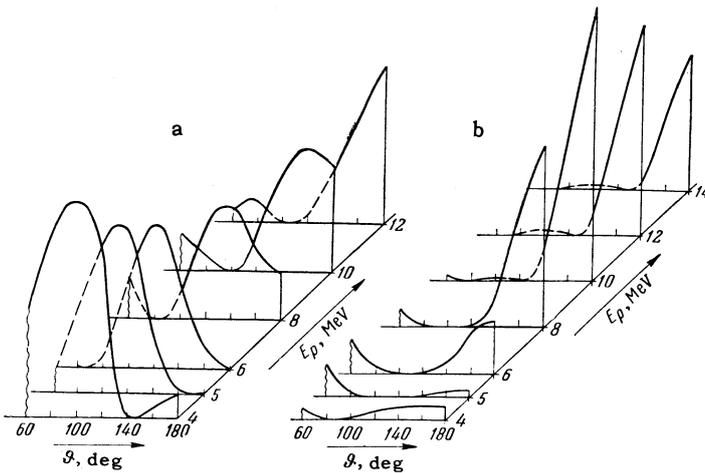
FIG. 2. Angular distributions of  $\alpha$  particles for the  $F^{19}(p, \alpha)O^{16}$  reaction for the following values of the parameters: a)  $R_0 = 4.8 F$ ,  $\rho_0 = 5.7 F$ ; b)  $R_0 = \rho_0 = 4.8 F$ .
