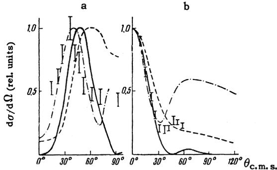
Angular distribution of protons, computed for three interaction variants, for the reaction  $Si^{30}(d, p)Si^{31}$  with formation of the  $Si^{31}$  nucleus a) in the ground state,  $l=2$ ; b) in the first excited state (0.76 Mev),  $l=0$ . The experimental points are from data of [1], the solid line is the Butler theory; the dashed line includes Coulomb interaction; the dot-dashed curve includes both Coulomb and nuclear interactions.
