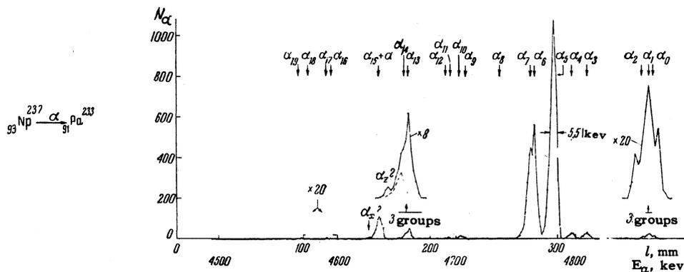
FIG. 1. Apparatus spectrum of the fine structure of  $\alpha$  radiation of Np<sup>237</sup>.
