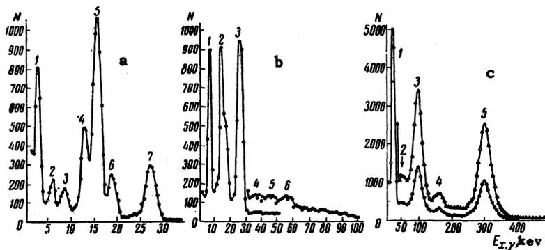
FIG. 2. X-ray and soft  $\gamma$ -ray spectrum of Ac<sup>227</sup>, obtained with the aid of a proportional counter: a) counter filled with mixture of Kr and CH<sub>4</sub>, b) counter filled with mixture of Xe and CH<sub>4</sub>, c) x-ray and  $\gamma$ -ray spectrum of Ac<sup>227</sup>, obtained with scintillation spectrometer.
