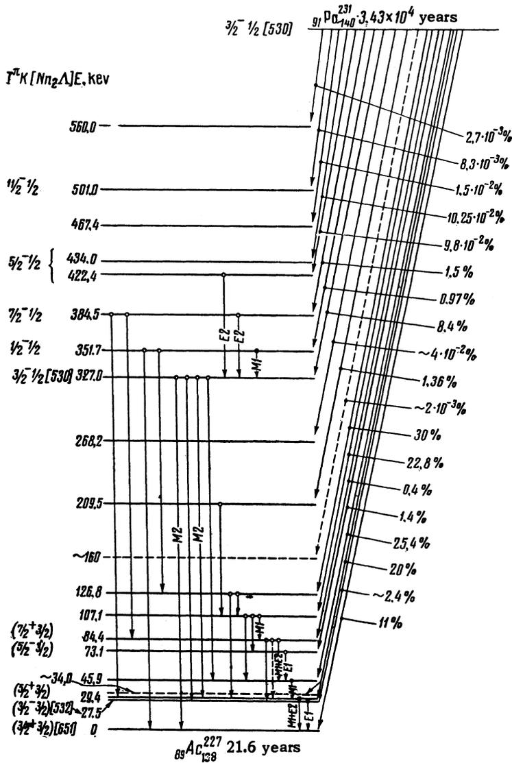
FIG. 3. Level scheme of  $\text{Ac}^{227}$ .
