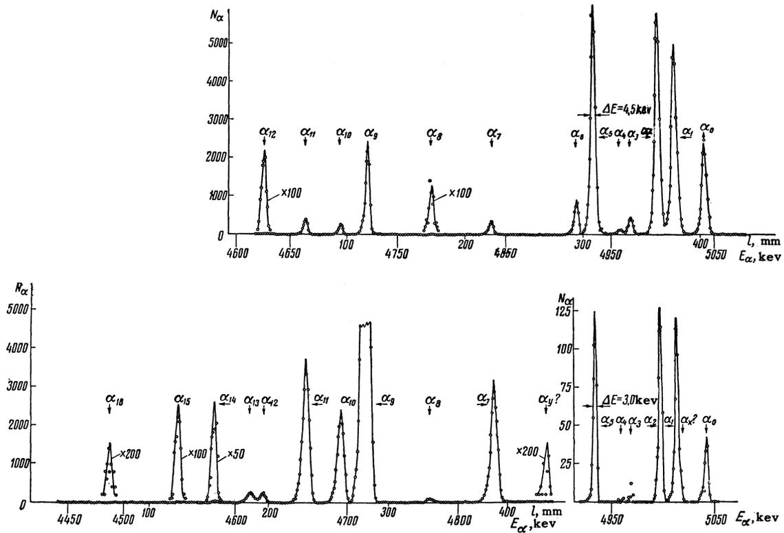
FIG. 1. Apparatus spectrum of the fine structure of the  $\alpha$  radiation of  $\text{Pa}^{231}$ .
