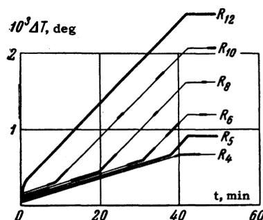
FIG. 3. Time dependence of thermometer temperatures for a thermal current in quiescent helium ( $W = 4.4 \times 10^{-2}$  w/cm<sup>2</sup>,  $T = 1.34^\circ\text{K}$ ).
