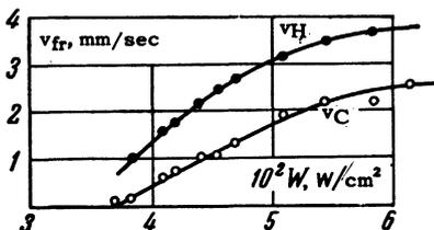
FIG. 4. Dependence of front velocity upon thermal current density ( $T = 1.34^\circ\text{K}$ ).
