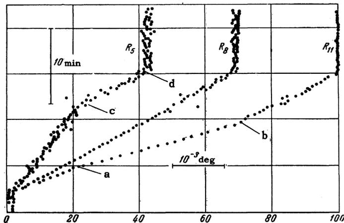
FIG. 5. Diagram of temperature readings as recorded by an EPP09-M1 for fronts propagating from ends and center of capillary.
