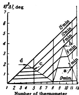
FIG. 6. Temperature distribution, relative to bath temperature, along the capillary. The spacing of the thermometers along the capillary is indicated on the x axis.
