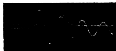
FIG. 6. Oscillogram of light pulse from plasma moving in a vacuum, phased with the current in the discharge chamber.
