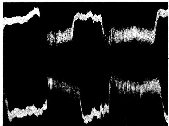
FIG. 8. Oscillograms of anode current (below) and discharge-chamber current (above) in a low-voltage discharge.  $I_d = 1$  amp;  $V_d = 15$  v;  $T = 300 \mu\text{sec}$ .
