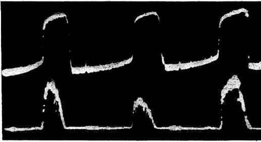
FIG. 9. Oscillations of anode current (top) and discharge-chamber current (bottom). Deflection upward corresponds to an increase in the electron current;  $T = 300 \mu\text{sec}$ ;  $\tau = 0.1 \mu\text{sec}$ ;  $A = 2.1 \text{ amp}$ ;  $I_d = 2 \text{ amp}$ ;  $V_d = 200 \text{ v}$ ;  $I_{av} = 1 \text{ amp}$ ;  $H = 1800 \text{ oe}$ ;  $L = 100 \text{ cm}$ ;  $p = 3 \times 10^{-6} \text{ mm Hg}$ .
