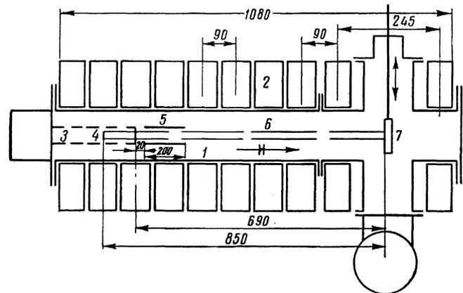
FIG. 1. Experimental apparatus: 1 - vacuum, 2 - solenoid, 3 - plasma source, 4 - cathode of source, 5 - filter, 6 - beam, 7 - anode. The dimensions are in millimeters.
