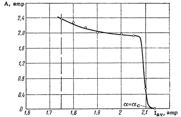
FIG. 10. Dependence of  $A$  on the concentration of the plasma at  $l = 2 \text{ cm}$ ,  $I_d = 2 \text{ amp}$ ,  $V_d = 120 \text{ v}$ ,  $H = 1800 \text{ oe}$ .
