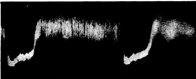
FIG. 6. Dependence of the anode current on the time. Upward deflection corresponds to an increase in the electron current.  $T = 500 \mu\text{sec}$ ;  $\tau = 0.15 \mu\text{sec}$ ; peak-to-peak oscillation  $A = 2$  amp;  $I_d = 1.8$  amp;  $V_d = 180$  v;  $I_{av} = 1$  amp;  $H = 1800$  oe;  $p = 4 \times 10^{-6}$  mm Hg;  $L = 100$  cm.
