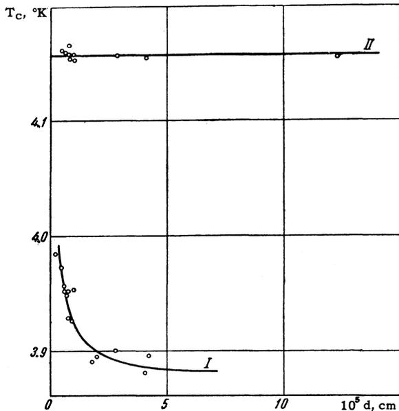
FIG. 3. The dependence of the transition temperature of a film on its thickness: I – freshly deposited films, II – annealed films.
