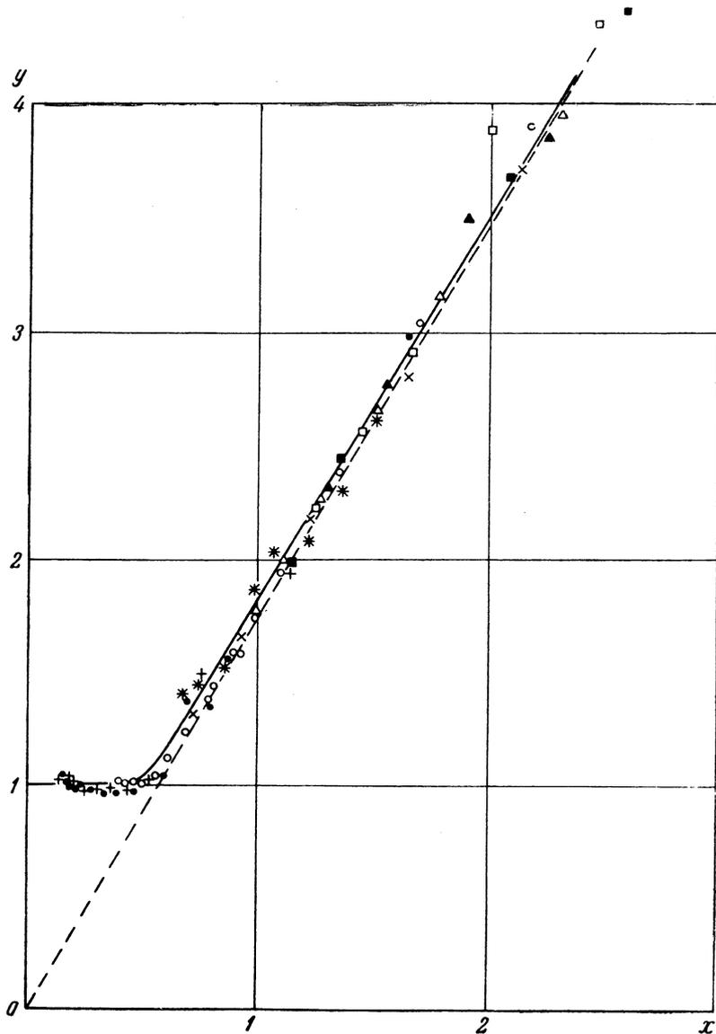
FIG. 5. The dependence of  $y = H_c/2\theta^2$  on  $x = 2.57 \times 10^{-4}/\theta d$  for films of thickness (in  $10^{-5}$  cm): + - 4.2,  $\bullet$  - 4.0,  $\circ$  - 2.8, \* - 1.0,  $\times$  - 0.9,  $\blacksquare$  - 0.83,  $\square$  - 0.81,  $\triangle$  - 0.76,  $\blacktriangle$  - 0.72. Full line is the theoretical curve.
