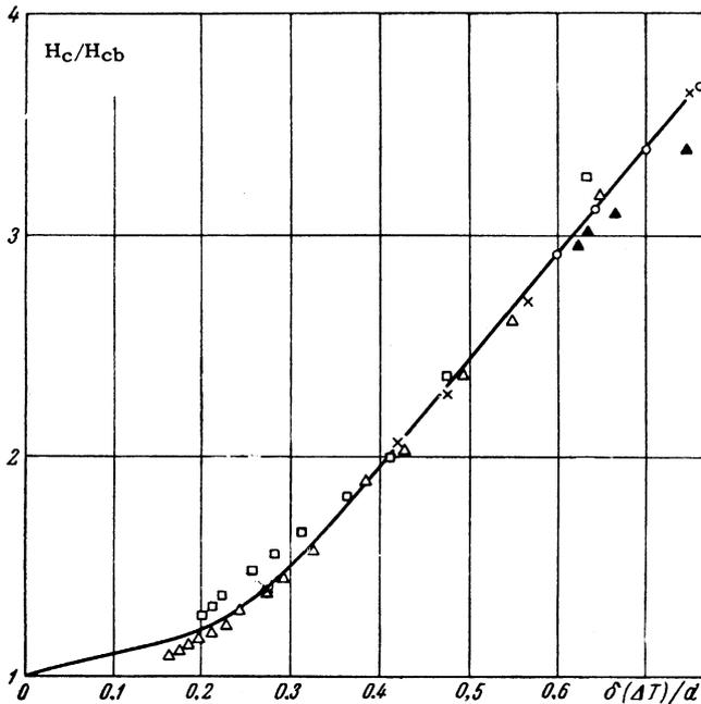
FIG. 6. The ratio  $H_c/H_{cb}$  as a function of  $\delta(\Delta T)/d$ . Film thickness in  $10^{-5}$  cm:  $\Delta$  - 4.9,  $\square$  - 4.1,  $\times$  - 2.8,  $\circ$  - 1.0,  $\blacktriangle$  - 0.9. The continuous curve shows the theoretical relation.
