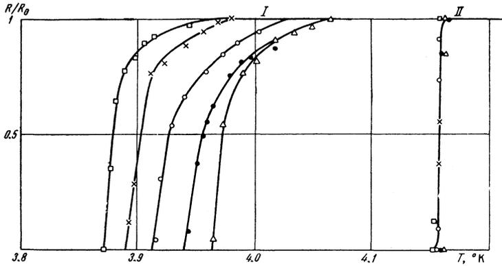
FIG. 2. The temperature dependence of the resistance of the films: I – freshly deposited films, II – annealed films. Film thicknesses in  $10^{-5}$  cm:  $\Delta$  – 0.46,  $\bullet$  – 0.58,  $\circ$  – 0.89  $\times$  – 2.8,  $\square$  – 4.0.
