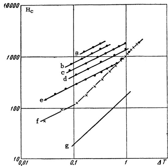
FIG. 4. The dependence of  $H_c$  on  $\Delta T$  ( $\Delta T = T_c - T$ ) for films of different thickness (in  $10^{-5}$  cm): a – 0.47, b – 0.58, c – 0.76, d – 0.90, e – 2.8, f – 4.2, g – bulk specimen.
