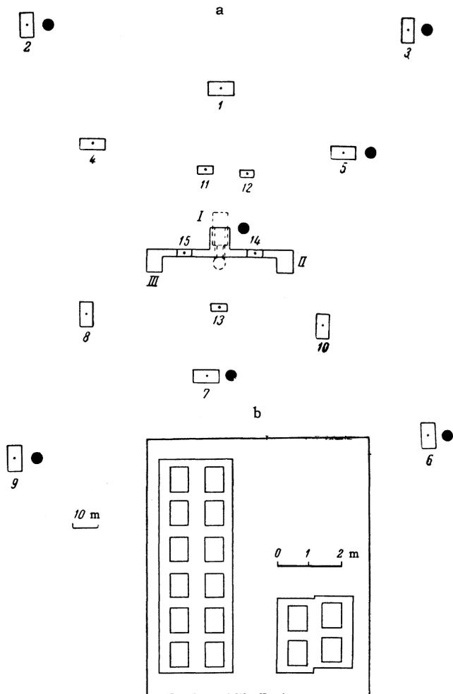
FIG. 1. a - position of the Geiger-Müller counter trays, ● -  $\mu$ -meson detectors; dashed line - outline of underground chambers; b - positions of detectors in the underground chamber U<sub>2</sub>. The squares indicate the effective areas of the counter groups.
