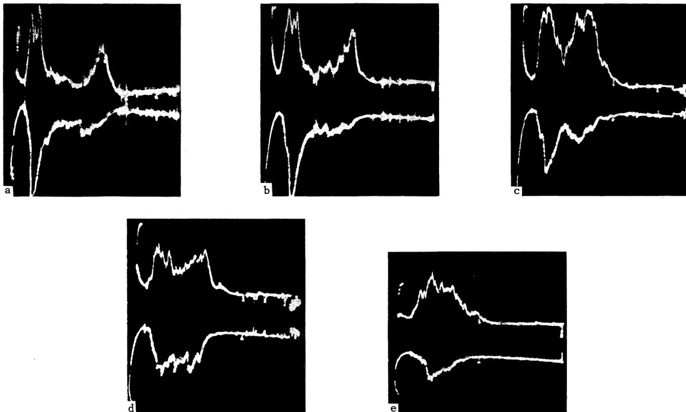
FIG. 3. Time dependence of the intensities of the OIII lines (upper trace) and OV lines (lower trace) for different values of the maximum discharge current: a— $I_{\max} = 120$  kAmp, b—95 kAmp, c—75 kAmp, d—65 kAmp, e—50 kAmp.
