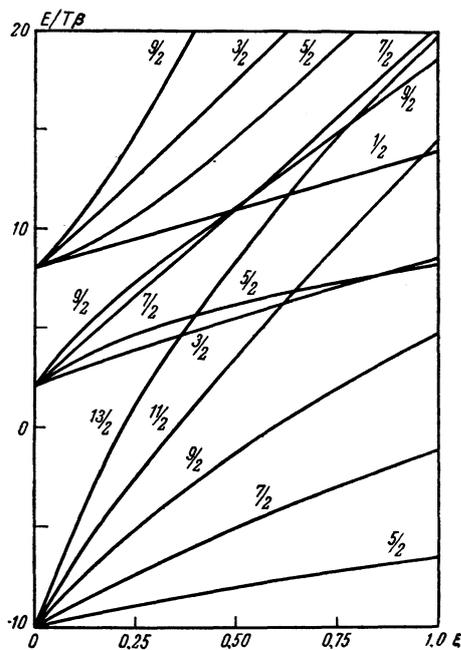
In using the figure, it is necessary to reckon the energy from the first line corresponding to a nuclear ground-state spin  $5/2$ . When  $\xi < 0.25$ , the spectrum of the excited states breaks up into three bands. The first band with spin sequence  $5/2, 7/2, 9/2, 11/2$ , and  $13/2$  can be called the "main rotational band." However, the rules governing the spacing of these levels differ from the rules derived from the adiabatic theory of rotational states for axially-symmetrical nuclei:
