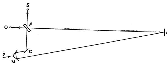
pattern, and M is a system of two mutually perpendicular plane mirrors which can be moved in the direction of the arrow with a controlled speed  $v$ .
