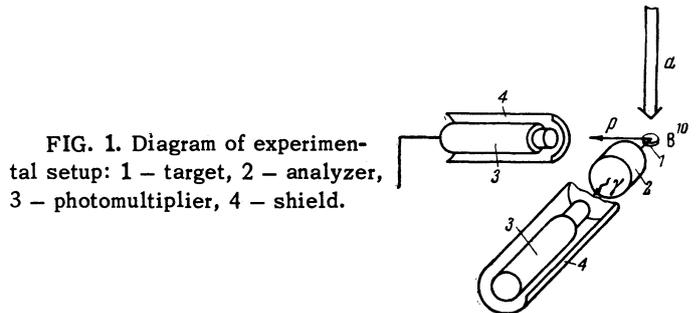
FIG. 1. Diagram of experimental setup: 1 - target, 2 - analyzer, 3 - photomultiplier, 4 - shield.
