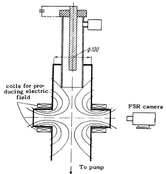
FIG. 4. Diagram of the magnetic trap designed for ultrahigh-speed movie photography of injection, capture, and plasma containment.
