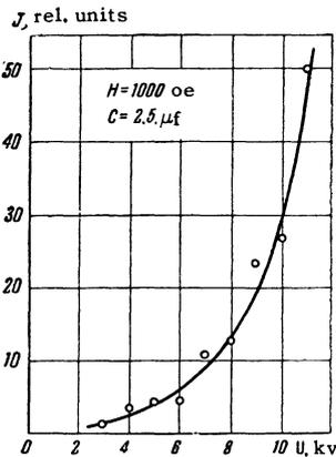
FIG. 2. The saturation ion current J as a function of the initial injector voltage U.
