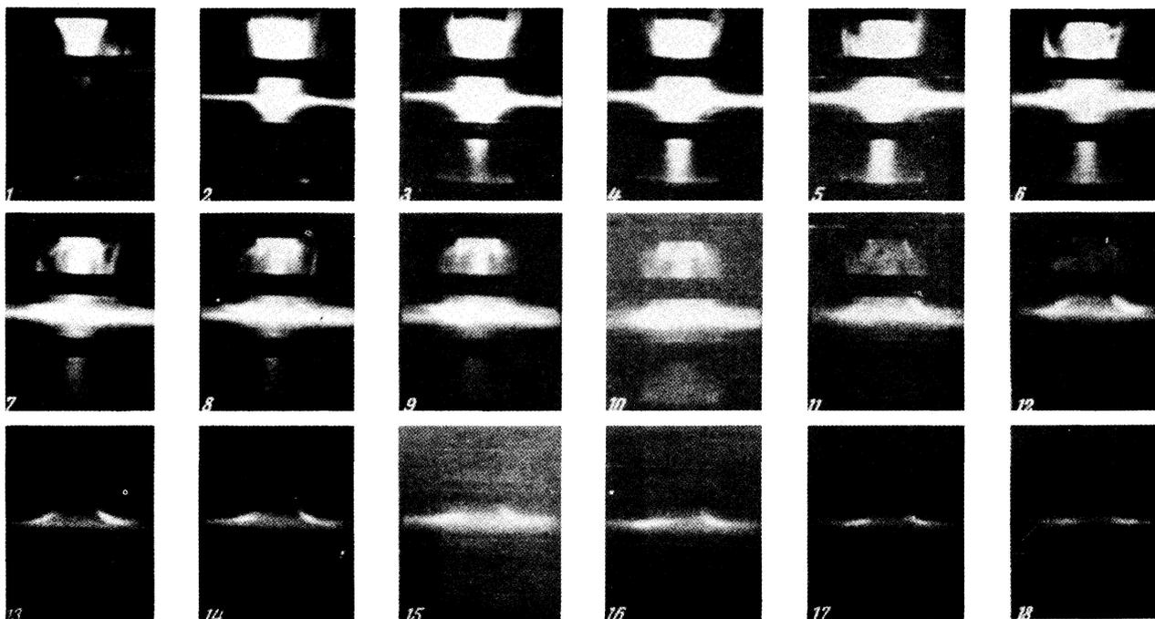
FIG. 5. Results obtained by ultrahigh-speed movie photography of the plasma with a magnetic trapping field. "Normal" plasma behavior. The time interval between frames is  $4 \mu\text{sec}$ .
