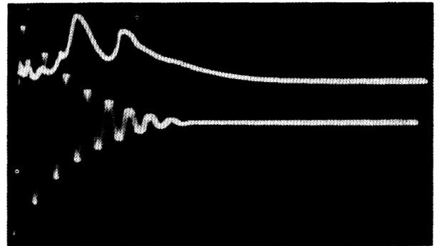
FIG. 3. The upper trace is the ion probe current with no magnetic trapping field. The lower trace is the current in the injector circuit. The sweep length is approximately 75  $\mu$ sec.
