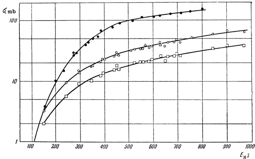
FIG. 1. Cross sections for the  $\text{He}^3 + \text{H}^3$  reaction as a function of triton energy  $E_{\text{H}^3}$ ; ● — total cross sections after Moak<sup>2</sup>; □ — cross sections for neutron branches; ○ — total cross sections obtained from the cross sections for the neutron branches and the ratio between the various reaction branches; △ — total cross sections obtained by counting charged particles.
