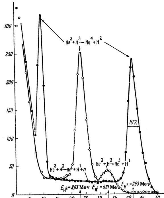
FIG. 2. Energy spectrum of particles from the  $\text{He}^3 + \text{H}^3$  reaction for  $E_{\text{H}^3} = 506$  keV: ● — total spectrum; ○ — the same spectrum after passing through an aluminum foil  $59.08$  mg/cm<sup>2</sup> thick. The abscissa gives the number of the channel in the analyzer, and the ordinate the relative number of counts per unit energy range (arb. units).
