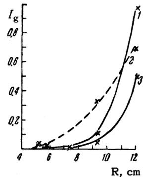
FIG. 2. Discharge in hydrogen,  $p = 0.05$  mm Hg. Curves 1, 2, and 3 are for the first, second, and third half cycles, respectively.
