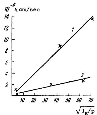
pendence of the speed of motion of the glowing rings on the gas pressure ( $v \sim p^{-1/2}$ ) agrees with the results of experiments on shock waves.<sup>3</sup>
