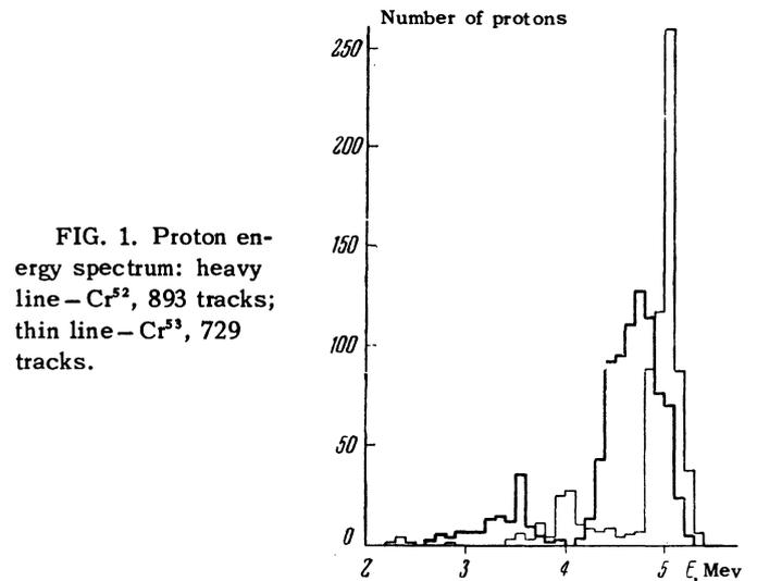
FIG. 1. Proton energy spectrum: heavy line -  $Cr^{52}$ , 893 tracks; thin line -  $Cr^{53}$ , 729 tracks.
