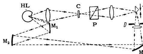
FIG. 3. Block diagram of the optical part of the photoelectric set-up for measuring optical thicknesses.
