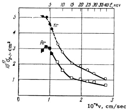
FIG. 1. Cross sections for electron capture by H atoms in argon and krypton. The dark points refer to the present work and the light points refer to the data of reference 1.
