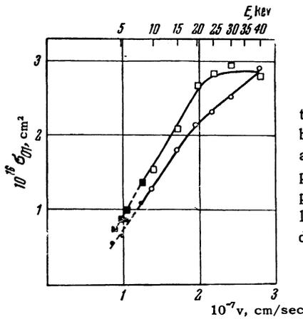
FIG. 7. Cross sections for electron loss by H atoms in argon and krypton. The dark points refer to the present work and the light points to the data of reference 1.
