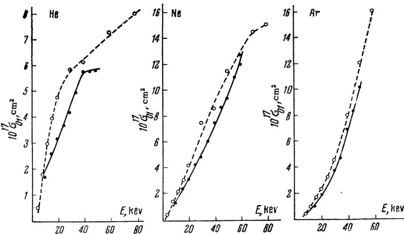
FIG. 11. The process He<sup>0</sup> → He<sup>+</sup>; ●) data of the present work, ○) data of reference 3.
