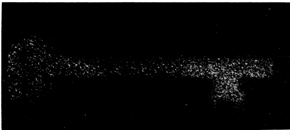
FIG. 3. Image of a key placed 20 cm in front of the chamber, with the chamber exposed through the glass window. The tube operated at 50 kv and 10 ma. The actual exposure was less than the sensitivity time of the chamber (on the order of a millisecond).
