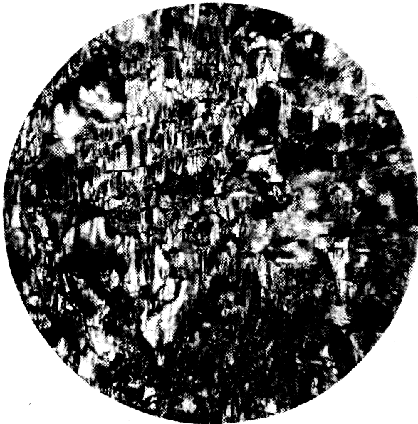
FIG. 6. Microrelief of copper surface after sputtering by hydrogen ions ( \times 130 ); a - E = 30 keV, j = 1.6 ma/cm 2 , t = 194 min; b - E = 14-54 keV, j = 0.07-0.8 ma/cm 2 , t = 842 min.
