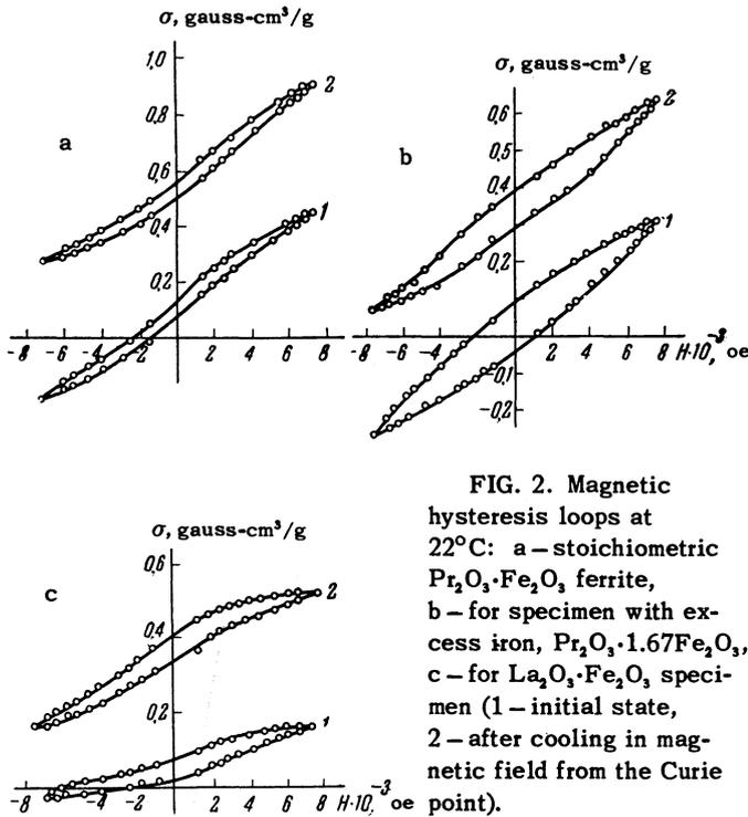
FIG. 2. Magnetic hysteresis loops at 22°C: a — stoichiometric  $\text{Pr}_2\text{O}_3 \cdot \text{Fe}_2\text{O}_3$  ferrite, b — for specimen with excess iron,  $\text{Pr}_2\text{O}_3 \cdot 1.67\text{Fe}_2\text{O}_3$ , c — for  $\text{La}_2\text{O}_3 \cdot \text{Fe}_2\text{O}_3$  specimen (1 — initial state, 2 — after cooling in magnetic field from the Curie point).
