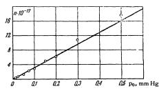
FIG. 2. The density of charged particles  $(n \sim \sqrt{1})$  measured at the time of maximum compression as a function of initial pressure in the chamber.
