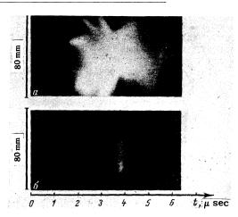
FIG. 1. Streak photograph of the discharge channel with spectrally resolved light at a pressure  $p_0 = 0.1 \text{ mm Hg: a}$  for the spectral region in the vicinity of  $H_{\alpha}(\Delta \lambda = 100 \text{ A})$ ; b) in the region  $\lambda = 6400 \text{ A} (\Delta \lambda = 100 \text{ A}, \text{ continuum})$ . The pictures were taken through a side window with which it was possible to view a portion of the discharge 8 cm in size.
