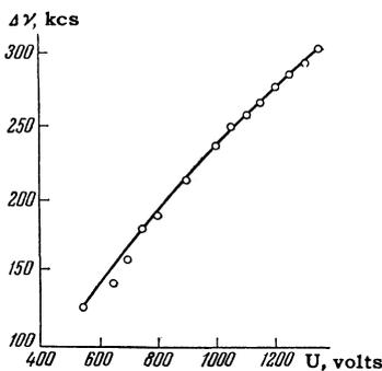
FIG. 9. Dependence of frequency on the potential of the cathode in the source.  $H = 1523$  oersteds;  $p \times 10^{-4}$  mm Hg.
