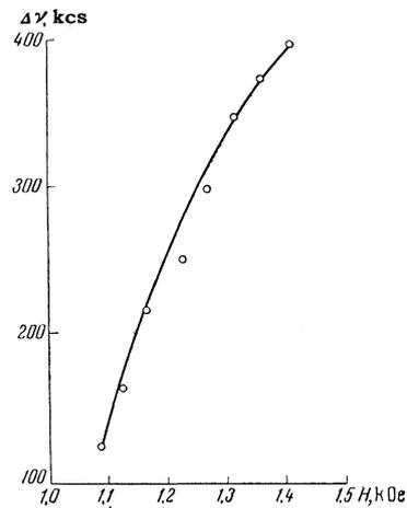
FIG. 10. Dependence of the frequency difference between neighboring lines on magnetic field.  $p = 5 \times 10^{-4}$  mm Hg.
