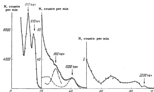
Gamma-ray spectrum of  $As^{74}$ , taken with a scintillation  $\gamma$ -ray spectrometer. The dashed curves show the resolution of a section of the spectrum into components.
