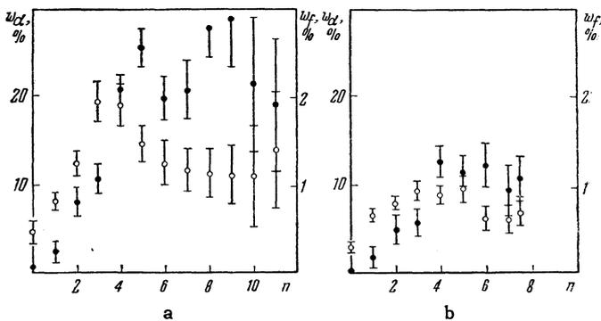
FIG. 5. The relative probability of emission of  $\alpha$  particles (light circles) and fragments (filled circles) and the dependence on the number of prongs in the star (H nuclei) for a – 660-Mev and b – 360-Mev protons.
