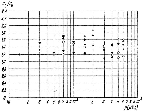
FIG. 4. The ratio of the deionization time constants in deuterium and in hydrogen  $\tau_D/\tau_H$  as a function of the pressure for  $\tau_0$  (initial) corresponding to  $\circ$ )  $d = 36$  mm,  $I_0 = 500$  ma;  $\bullet$ )  $d = 65$  mm;  $I_0 = 500$  ma;  $+$ )  $d = 65$  mm,  $I_0 = 60$  ma; for  $\tau_c$  (final) corresponding to  $\blacktriangle$ )  $d = 36$  mm,  $I_0 = 1500$  ma;  $\blacktriangledown$ )  $d = 65$  mm,  $I_0 = 1500$  ma;  $\times$ )  $d = 65$  mm,  $I_0 = 60$  ma.
