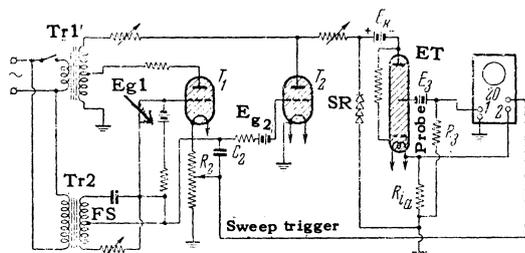
FIG. 1. Circuit for the measurement of the rate of deionization in hydrogen.
