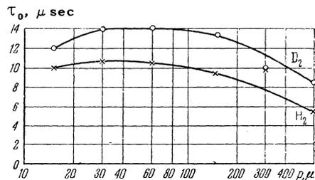
FIG. 3. The initial deionization "time-constant"  $\tau_0$  in  $D_2$  and in  $H_2$  as a function of the pressure;  $I_0 = 0.5$  amp,  $d = 65$  mm.
