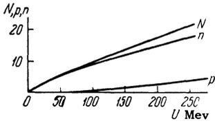
FIG. 7. Number of evaporated particles as a function of the excitation energy  $U$ :  $N$ ) total number of nucleons,  $n$ ) neutrons,  $p$ ) protons.
