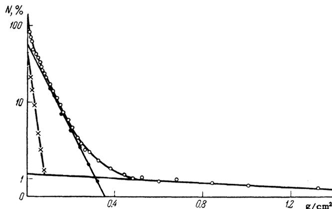
FIG. 2 o) absorption curve of total radiation from  $\text{Re}^{186}$  in aluminum; x) L radiation; ●) beta component; solid line – gamma background.
