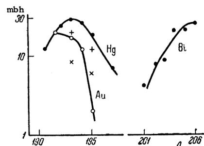
FIG. 6. Dependence of the cross section for the production of radioisotopes of gold, mercury, and bismuth on the mass number, at a proton energy of 660 Mev: +) yield of mercury radioisotopes in the ground state; x) the same in the isomer state; ●) total yield of radioisotopes of mercury and bismuth; ○) yield of gold radioisotopes.
