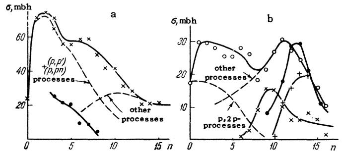
FIG. 8. Cross sections for disintegration as a function of the number of emitted neutrons  $n$  and the number of protons  $p$ : a) for  $p = 1$  ( $\times$  - calculated values,  $\bullet$  - experimental values for Bi); b) for  $p = 2$  ( $\circ$  - calculated values,  $\bullet$  - experimental data for Hg) and for  $p = 3$  ( $\times$  - calculated values,  $+$  - experimental data for gold).
