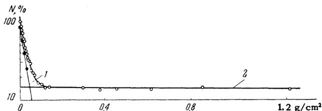
FIG. 1. Absorption curve for electromagnetic radiation from  $\text{Re}^{186}$  in aluminum: 1) L radiation; 2) gamma background ( $N$  is the number of counts as percentage of the initial count).
