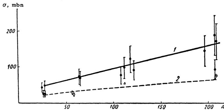
FIG. 2. Dependence of the tritium production cross section on the atomic weight of the target material at 1) 660 Mev and 2) 450 Mev.
