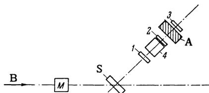
FIG. 1. Schematic diagram of the experiment.  $n$  - neutron beam,  $M$  - monitor (ionization chamber), 1, 2, 3 - scintillation counters, 4 - radiator of the Cerenkov counter,  $A$  - absorber,  $S$  - scattering medium.
