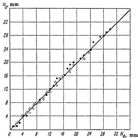
FIG. 3. Dependence of the equilibrium orientation  $N_d$  of the disk system upon the orientation  $N_f$  of the frame; i.e., the angle of twist of the fiber. Solid line — calibration curve. ● — measurements of 24 Dec., 1956; ○ — measurements of 18 Jan., 1957, Δ — measurements of 1 Feb., 1957.
