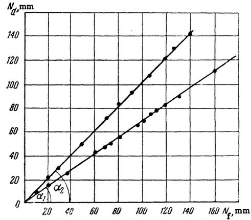
FIG. 2. Calibration curves:  $\tan \alpha_1 = \Delta N_d/\Delta N_f = 0.71 \pm 0.007$ ;  $\tan \alpha_2 = \Delta N_d/\Delta N_f = 1.03 \pm 0.01$ .
