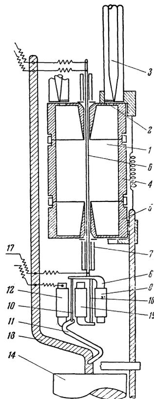
only the sample, which serves as part of the measuring resonator, is cooled to the temperature of the alum. The remaining parts of the apparatus are at the temperature of the helium bath ( $\sim 1.6^\circ\text{K}$ ).
