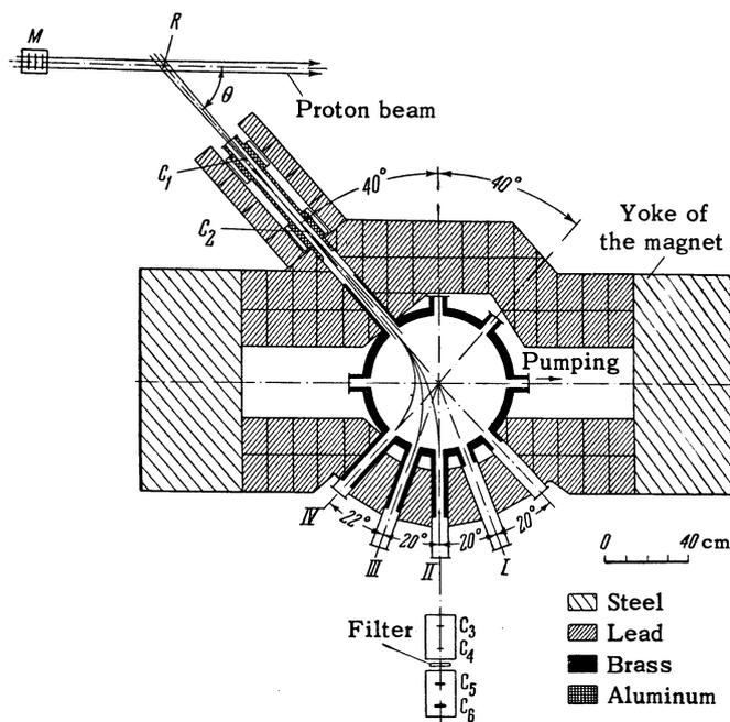
FIG. 2. Diagram of the spectrometer: M - monitor, R - target, C<sub>1</sub> to C<sub>6</sub> - scintillators.
