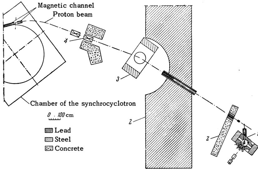
FIG. 1. Placement of the spectrometer (1), shielding wall (2), deflecting magnet (3), and focusing lens (4), shown relative to the synchrocyclotron chamber.
