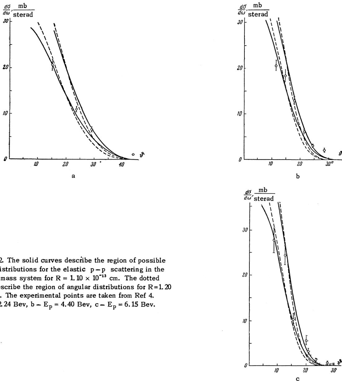
FIG. 2. The solid curves describe the region of possible angular distributions for the elastic p-p scattering in the center of mass system for  $R = 1.10 \times 10^{-13}$  cm. The dotted curves describe the region of angular distributions for  $R = 1.20 \times 10^{-13}$  cm. The experimental points are taken from Ref 4. a -  $E_p = 2.24$  BeV, b -  $E_p = 4.40$  BeV, c -  $E_p = 6.15$  BeV.
