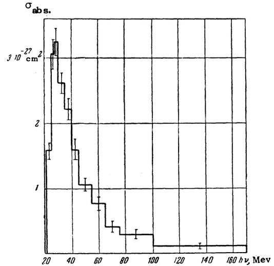
FIG. 8. Dependence of total cross section for absorption of photons by  $\text{He}^4$  on photon energy. Only statistical errors are shown on the graph. Errors in absolute values are  $\sim 6\%$ .
