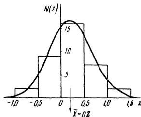
FIG. 5.  $p_{\perp}$  distribution of  $\pi^0$ -mesons obtained from the energy and angle of emission of electron pairs (data of Refs. 12, 14, and 11).  $N=36$ ,  $(\bar{p}_{\perp})_{\text{geom}} = 1.6 \mu c$ ,  $\sqrt{D(p_{\perp})}/\bar{p}_{\perp} = 1.0$ .
