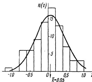
FIG. 4. Distribution of secondary particles with respect to  $p_{\perp}$  for  $E_0 \sim 5 \cdot 10^{12} \text{ ev}$ . Data of Ref. 5-7 and of the author (multiple scattering method, emulsion).  $N = 80$ ,  $(\bar{p}_{\perp})_{\text{geom}} = 1.1 \mu c$ ,  $\sqrt{D(p_{\perp})}/\bar{p}_{\perp} = 0.9$ .
