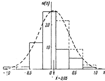
FIG. 2. Distribution with respect to  $p_{\perp}$  of secondary particles for  $\bar{E}_0 = 5 \text{ Bev}^3$  (cloud chamber method).  $N = 72$ ,  $(\bar{p}_{\perp})_{\text{geom}} = 1.1 \mu c$ ,  $\sqrt{D(p_{\perp})}/\bar{p}_{\perp} = 0.8$ .
