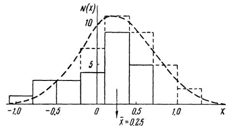
FIG. 3. Distribution of secondary particles with respect to  $p_{\perp}$  for  $E_0 = 30 \text{ Bev}^4$  (cloud chamber method).  $N = 41$ ,  $(\bar{p}_{\perp})_{\text{geom}} = 1.8 \mu c$ ,  $\sqrt{D(p_{\perp})}/\bar{p}_{\perp} = 1.0$ .
