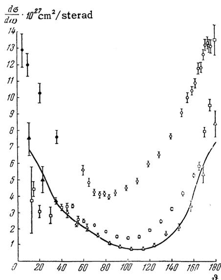
FIG. 2. Differential cross section for elastic n-p scattering. ●, ○ - Ref. 5,  $E_n = 91$  Mev; □ - Ref. 4,  $E_n = 400$  Mev; △ - Ref. 1,  $E_n = 580$  Mev; ▲ - Present work. Solid curve - graph of the approximate expression (3).
