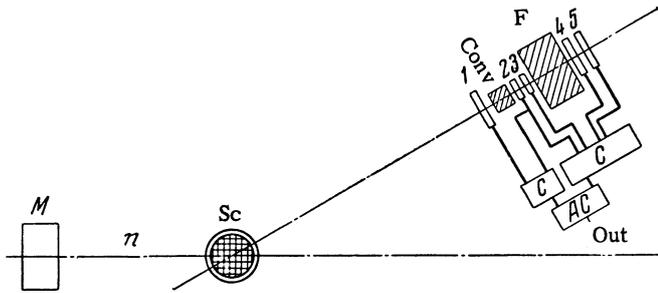
FIG. 1. Experimental arrangement.  $n$  – neutron beam; M – monitor; Sc – scatterer (Dewar flask with liquid hydrogen); 1, 2, 3, 4, 5: scintillation counters; Conv – converter; F – filter; C – coincidence arrangement; AC – anticoincidence arrangement; Out – output.
