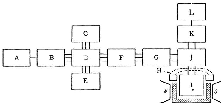
FIG. 1. Block diagram of the klystron oscillator. A) ferromagnetic resonance stabilizer; B) electronic stabilizer; C) power monitor; D) oscillator; E) resonance wave meter; F) variable attenuator; G) choke joint; H) cooling system; I) absorption cell; J) heater; K) detector; L) recorder.
