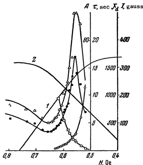
FIG. 2. 1, the back of the hysteresis loop,  $I$ ; 2, curve of the differential susceptibility,  $\chi_d$ ;  $\Delta$  and  $\bullet$ —curves of viscosity,  $\tau_{0.05}$  and  $\tau_{0.01}$ ;  $\circ$ —curve of the time of appearance of the second maximum of  $\tau$ ;  $\square$ —amplitudes of the second maximum  $A$  for specimen 4.
